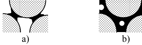
Fig. 6 Residual fluid content: Wetting (black) and non-wetting fluid (white) in a porous medium consisting of mineral solid (grey); a) wetting fluid residual content; b) non-wetting fluid residual content (schematic).
